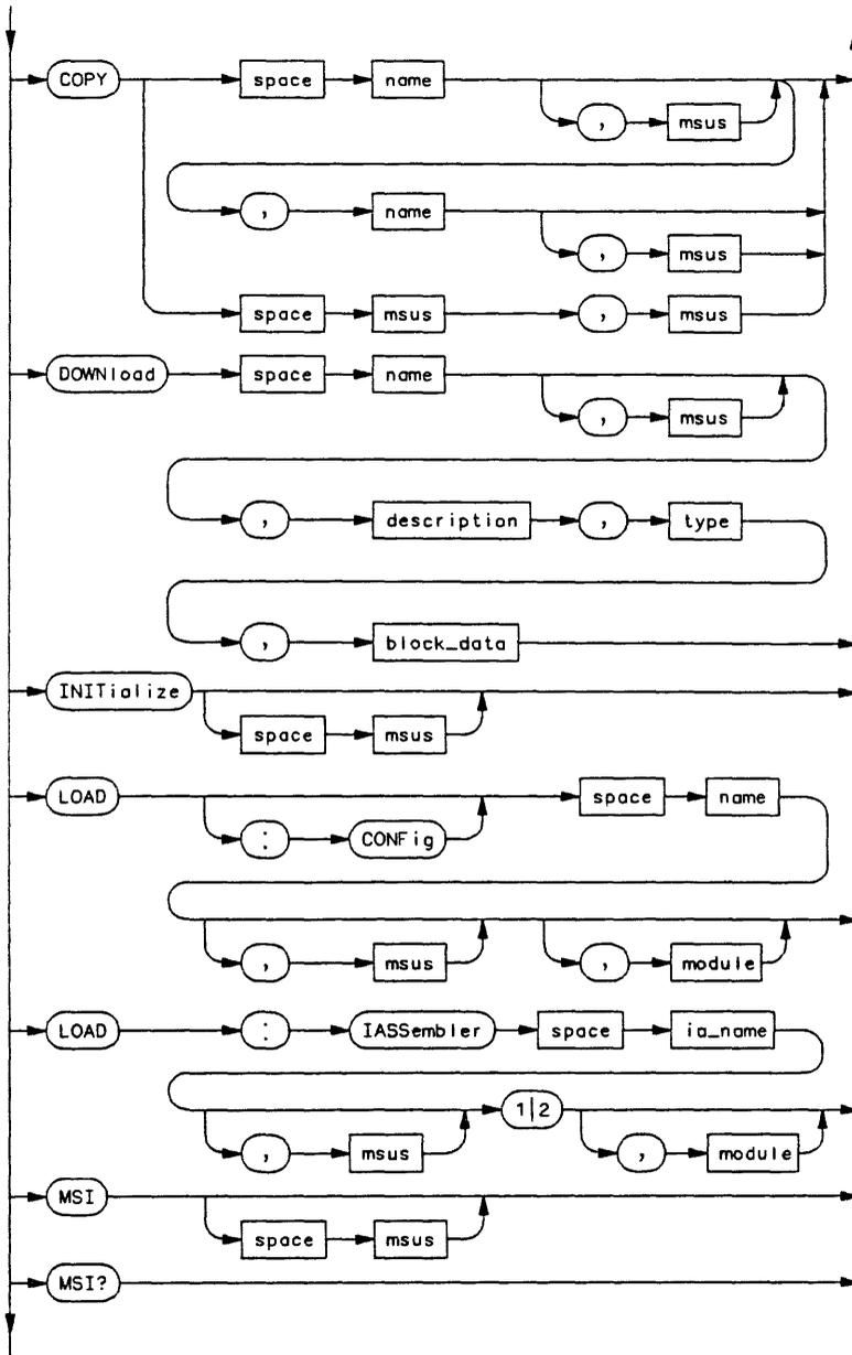
Figure 8-1. Mmemory Subsystem Commands Syntax Diagram (Continued)
