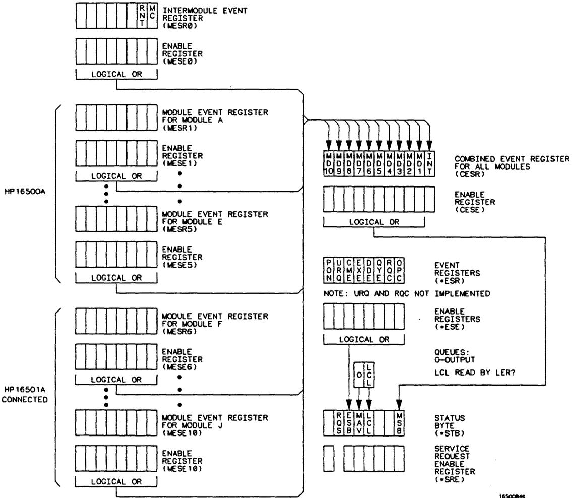
Figure B-1. Status Byte Structures and Concepts
