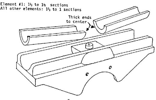
butts are flush and mounting holes are aligned. Lay the element half butt into the insulator channel. Insert  $10-32 \times 2 \cdot 1/2$ " screws from bottom of insulator and secure above element butt with 10-32 nuts and lockwashers. Holes in element half butt will align one way only (drilled slightly off square to compensate for element "lift" designed into insulator). If screws are not an easy fit, rotate element half butt 180 degrees and repeat.
