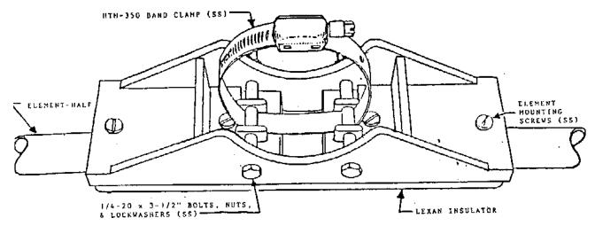
\*IMPORTANT NOTE: The INSULATOR is made of LEXAN plastic, which is one of the toughest materials available,...strong and firm,...flexible but not brittle. It does not expand or contract with heat or cold (+-.005) However, the metal fasteners that you use with this insulator change in size with temperature variances.
