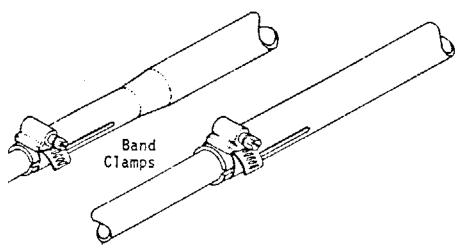
D. The chart below lists the tubing lengths supplied for each element half, the proper band clamp for each overlap, and the correct element half length (adjust the tip section). Remember to use Penetrox at each overlap and securely tighten clamps until tubing cannot be pulled out or rotated. Pair up element halves as they are completed to avoid mixups.
