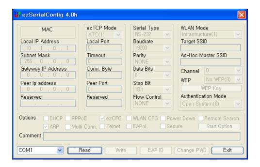
Operate EZL-80c in serial configuration mode to utilize ezSerialConfig. Follow the sequence as described below.
