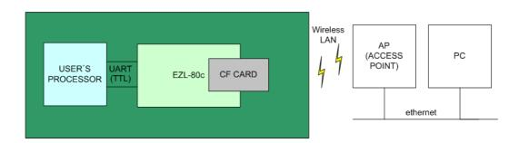
EZL-80c is a small-sized, modular product that provides TCP/IP communication through IEEE802.11b (wireless LAN) among the ezTCP product group and has a CF card socket and requires a 16-bit CF wireless LAN card.
